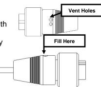
Figure 1 – CC-AXX & JXX with Injection Vent Holes
