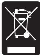
Fig. 1.4: Product labeling in accordance with EN 50419
